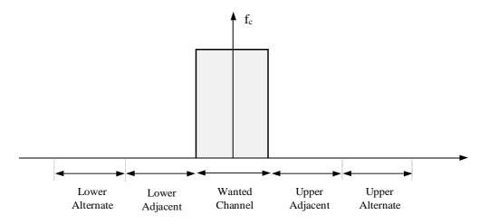
Figure 1: Adjacent and alternate channel definitions
