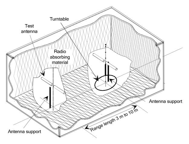
Figure B.1: A typical anechoic chamber
