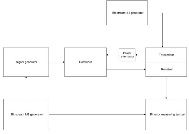
Figure 9: Measurement arrangement
