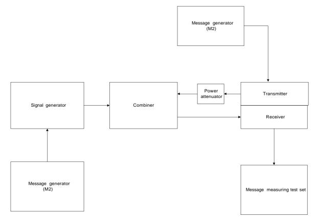
Figure 11: Measurement arrangement
