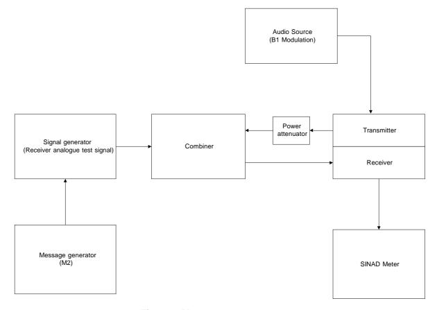
Figure 7: Measurement arrangement
