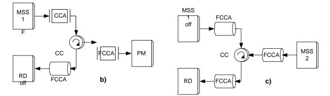
Figure B.6: Measurement arrangement with one antenna connector: a) for measurement of EUT parameters b) for adjusting input power to EUT c) for substitution measurements
