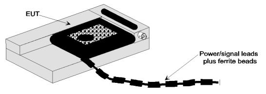
Figure B.5: EUT mounted in a typical test fixture
