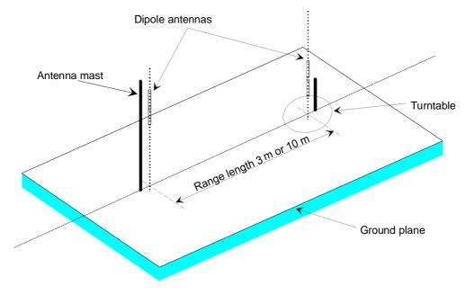
Figure B.3: Typical open area test site
