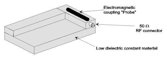
Figure B.4: Typical test fixture
