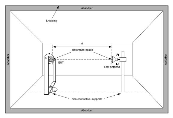
Figure B.1: Typical anechoic chamber
